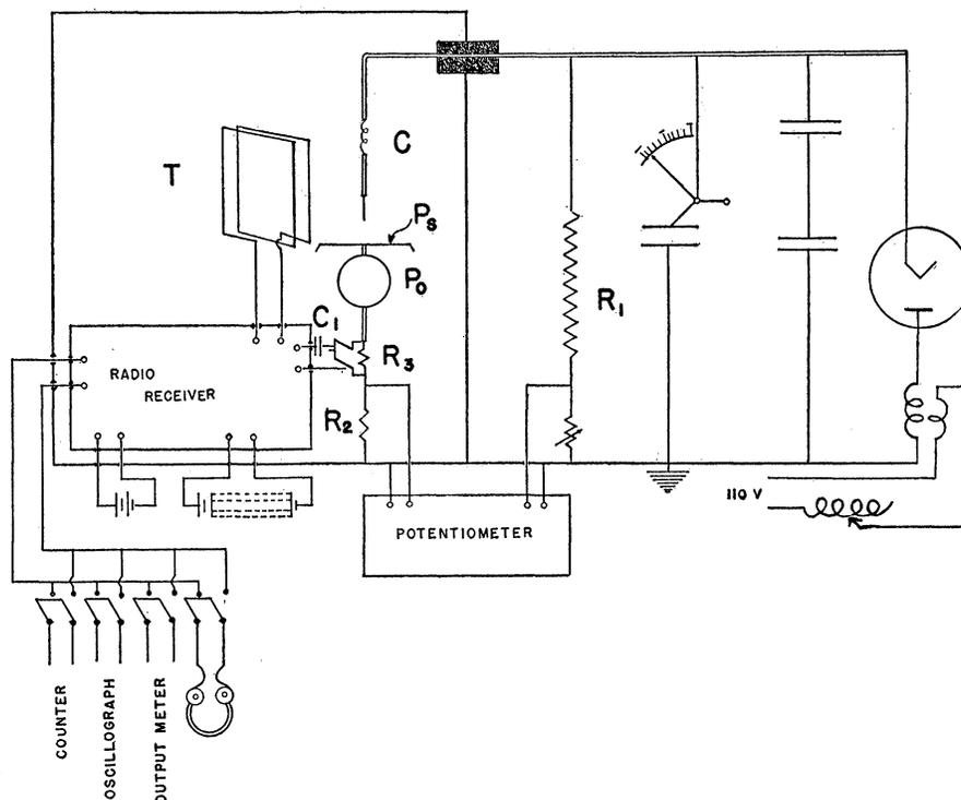
FIG. 1. Diagram of connections used in the study of positive point-to-plane corona.
