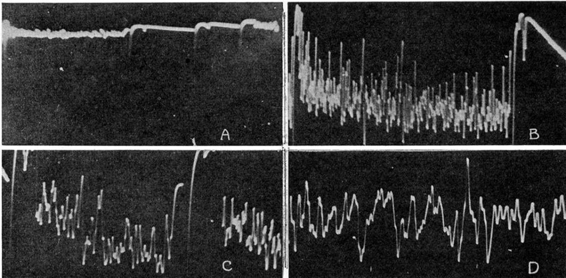
FIG. 2. *A*. Oscillogram of an intermittent positive corona for a current near onset with low magnification. Steady current is 20 to 40 times the amplitude of the oscillations. *B*. Same as *2A* with large amplification and slower sweep. *C*. Same as *2A* with larger amplification and the same sweeping rate. *D*. Oscillogram of a section of stable positive corona at 62,500 resolved fluctuations per second, at  $1\mu A$  current.
