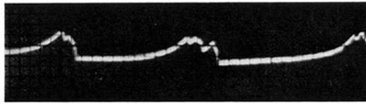
FIG. 8. Oscillograph by Kip showing the intermittent corona just below onset. Three intermittent discharges are seen. The fluctuations cannot be clearly resolved. The sweep is from right to left and the time covered in the oscillogram is 0.015 sec. The asymptotic decline to the left is instrumental.
