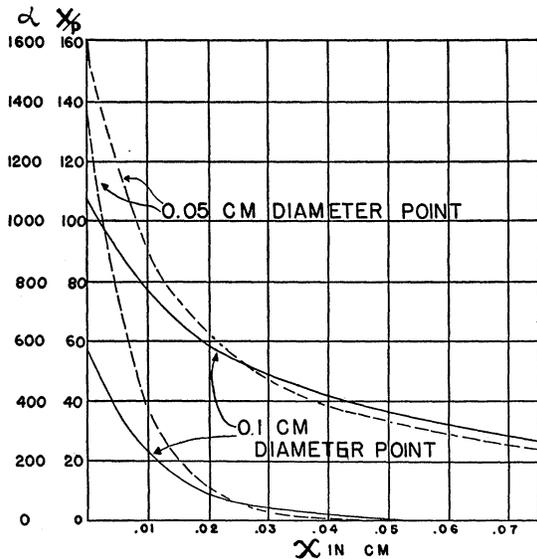
FIG. 4. Field strength divided by pressure,  $X/p$ , after Kip and Townsend's coefficient  $\alpha$  for ionization by electron impact in air after Sanders as a function of distance from point for 0.05 (dashed) and 0.1 (full) cm diameter points at starting potentials for positive corona. The curves above give the values of  $X/p$ . Those asymptotic at about 0.04 cm give the values of  $\alpha$ .
