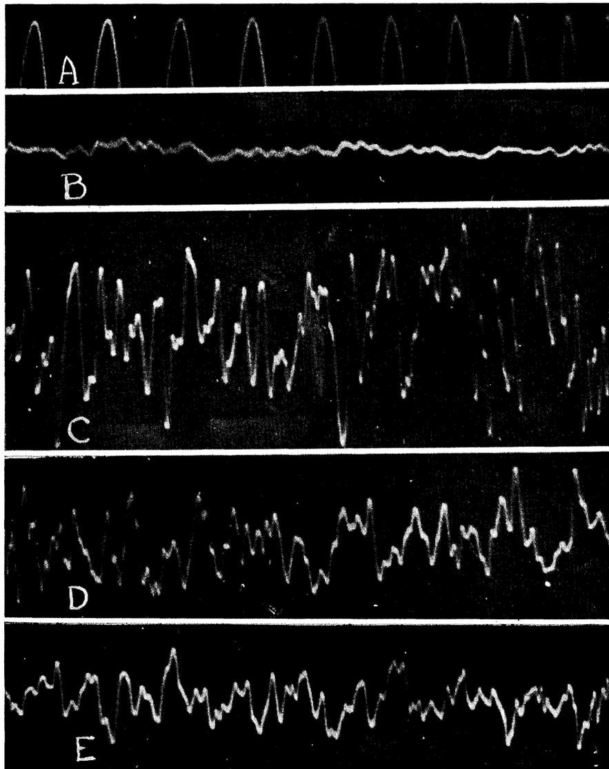
FIG. 3. *A.* An 8000 cycle per second timing wave. *B.* Parasitic background oscillations with full gain on the amplifier and no corona. *C.* Corona with 0.5-mm diameter point, current  $0.5\mu\text{A}$ . *D.* Same as *C* current  $1\mu\text{A}$ . *E.* Same as *C* current  $2\mu\text{A}$ .
