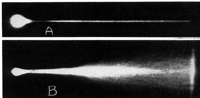
FIG. 7. *A*. Photograph of the positive point corona just before the appearance of streamers. A few incipient streamers may be seen beyond the edge of the glow. Potential 20.0 kv. *B*. Photograph of streamers propagating across the gap shortly after streamer onset. The cathode is distinguished by the glow over its surface. Potential 21.5 kv.
