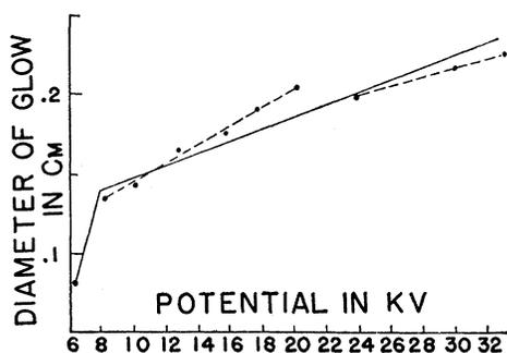
FIG. 6. Plot of the diameter of the glow of the positive point corona as the potential increases.
