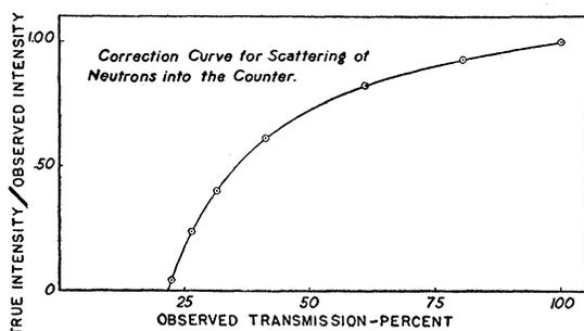
Fig. 1. Correction curve for scattering of neutrons into the counter.
