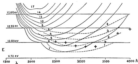
FIG. 7. Relations between  $I_\lambda$ ,  $\lambda$ , and energy of exciting electrons  $E$ , for  $H_2$ . Lines of constant  $I_\lambda$  (—). Lines of constant illumination of plate in quartz spectrograph (- - -). Data of Finkelberg and Weizel (+ +). Intensities in arbitrary units.
