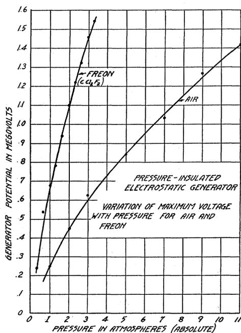
FIG. 4. Increase of generator voltage with pressure for air and Freon.
