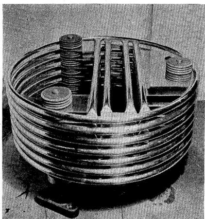
FIG. 2. View of partially assembled generator column.
