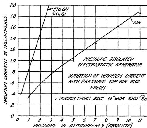
FIG. 3. Increase of generator current with pressure for air and Freon.
