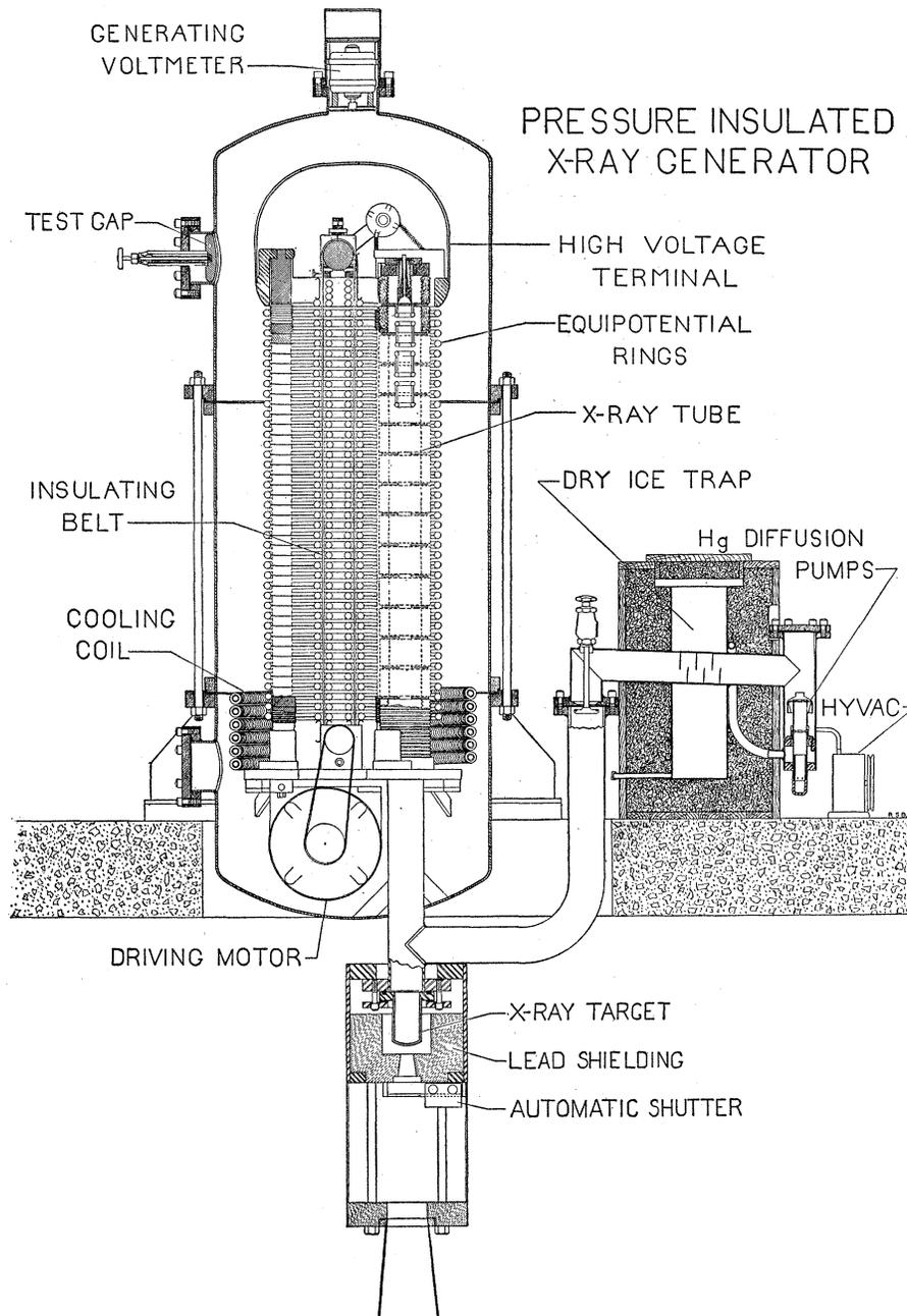
FIG. 1. Sectional view of pressure-insulated x-ray generator.
