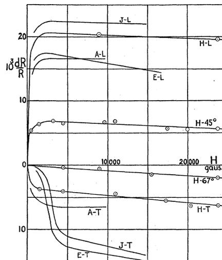
FIG. 1. Magnetoresistance of nickel as a function of magnetic field. Curves from various authors are indicated as follows: *J*, Jones and Malam; *H*, Heaps; *A*, Alocco; *E*, Englert. The letters *L* and *T* indicate longitudinal and transverse fields, respectively.
