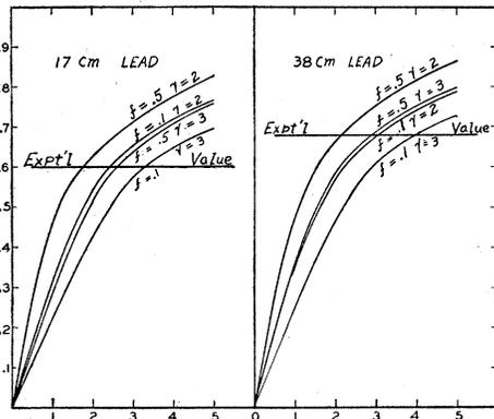
FIG. 1. Ordinates: calculated values of  $j_\zeta/j_v$ . Abscissae: the rest life  $\tau_0$  in microseconds.
