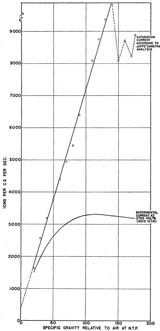
FIG. 3A. "Saturation" current curve corresponding to our observations with central-source, together with experimental curve obtained with strongest collecting field.
