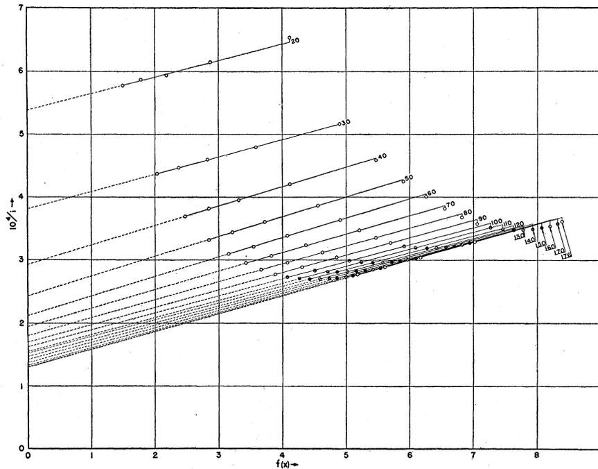
FIG. 2A. Jaffé-Zanstra function curves corresponding to our measurements with ring-source. Air at 27°C. Ring-source of gamma-radiation beneath chamber. Numbers at upper ends of curves represent specific gravity relative to air at N. T. P.
