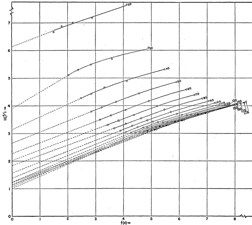
FIG. 1A. Jaffé-Zanstra function curves corresponding to our measurements with central-source. Air at 28°C. Central source of gamma-radiation. Numbers at upper ends of curves represent specific gravity relative to air at N. T. P.
