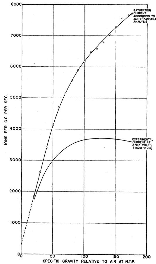
FIG. 4A. "Saturation" current curve corresponding to our observations with ring-source, together with experimental curve obtained with strongest collecting field.
