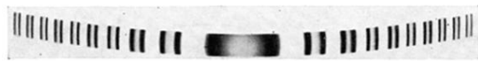
FIG. 1. Interferometer fringes of H and D obtained with a 3-mm étalon spacing.
