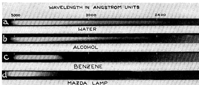
FIG. 4. Spectra of Čerenkov radiation produced in liquids by high velocity electrons. 1 mm slit, exposures 10 minutes.
