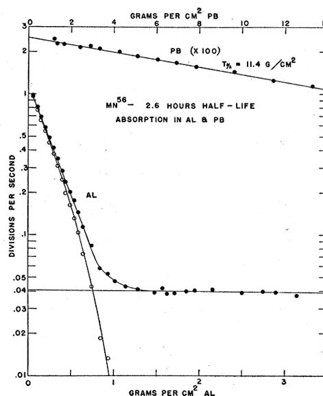
FIG. 10. Absorption curves of  $\text{Mn}^{56}$ .
