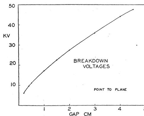
Fig. 6. Breakdown voltage vs. gap distance, hemispherical point.
