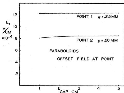
Fig. 5. Field at point surface at onset for confocal parabolic electrodes for various gap distances.
