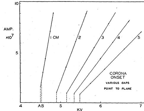
FIG. 2. Onset region of corona current-voltage curves, enlarged, showing initial linear current rise.
