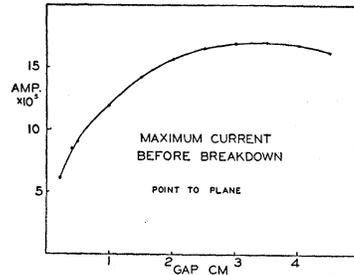
FIG. 7. Maximum current before spark breakdown vs. gap distance.
