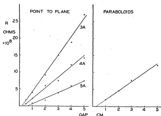
FIG. 8. Effective resistance interposed by clearing field region of gap vs. gap distance for point to plane and parabolic gaps. Point 3A, diameter 0.5 mm; point 4A, diameter 1.5 mm; point 5A, diameter 4.7 mm.
