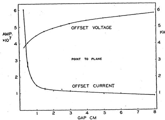
FIG. 3. Offset voltage and current vs. gap distance for hemispherical point 3A.
