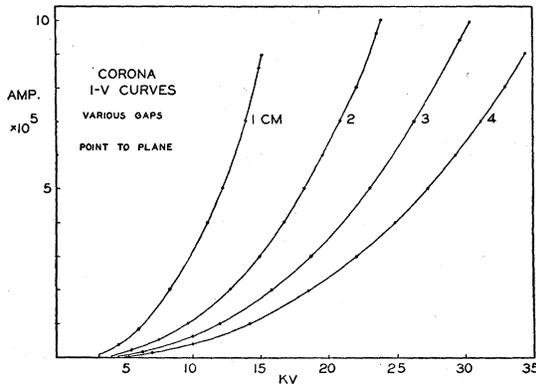
FIG. 1. Corona current-voltage curves for various gap distances. Curves end at voltage at which spark breakdown occurs. Hemispherical point 3A, diameter 0.5 mm.
