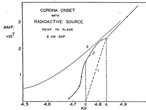
FIG. 4. Effect of radioactive source on corona onset, 2.0 cm gap, point 3A. Curve 1, weak source; curve 2, medium source; curve 3, strong source.
