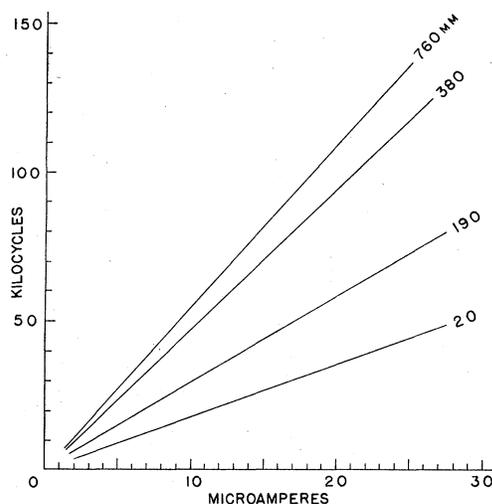
FIG. 5. Plot of the variation of frequency as a function of air pressure.
