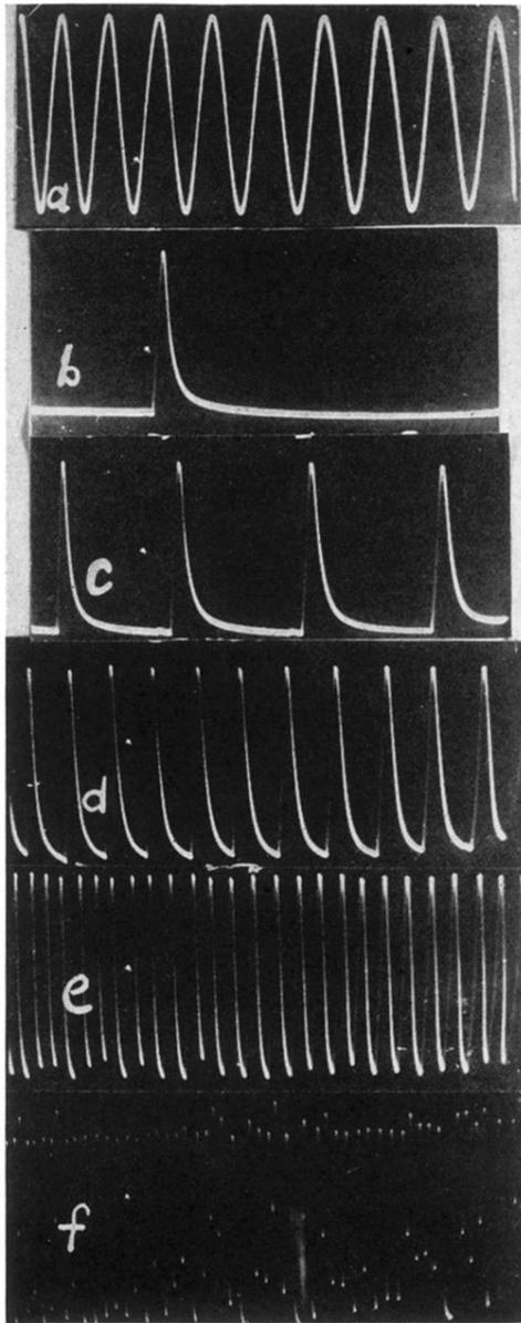
FIG. 2. Typical oscillograms of negative point corona for a 0.5-mm diameter point and 3-cm gap. (a) 8000 cycles calibrating wave; (b) single pulse  $0.1\mu\text{A}$ ; (c)  $0.7\mu\text{A}$ ; (d)  $2.0\mu\text{A}$ ; (e)  $5.0\mu\text{A}$ ; (f)  $12.0\mu\text{A}$ .
