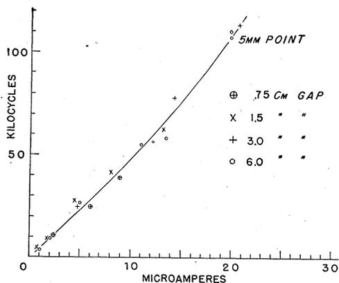
FIG. 4. Plot of the variation of frequency with change in gap distance for a 0.5-mm point.
