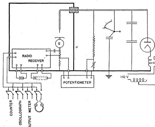
FIG. 1. Schematic diagram of the electrical circuits employed for negative point corona measurements.
