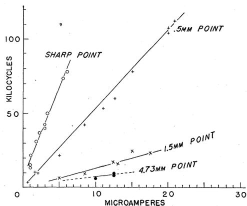
FIG. 3. Plot of the variation of frequency as a function of point size.
