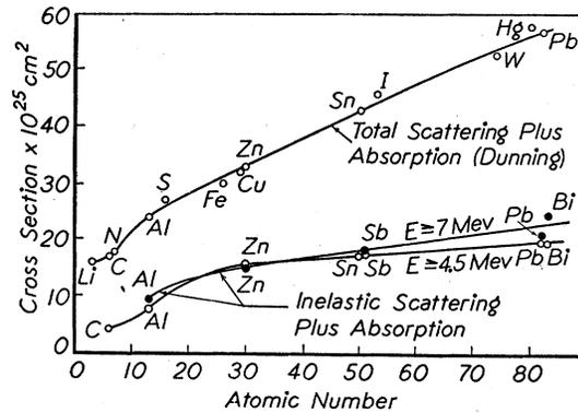
FIG. 1. Upper curve, total scattering+absorption cross sections for fast neutrons (Dunning). Lower curves, inelastic scattering+absorption cross sections for fast neutrons as measured with iron detectors ● or with aluminum detectors ○.
