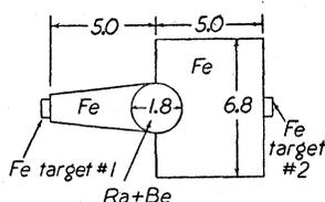
FIG. 2. Experimental arrangement for demonstrating scattering of fast neutrons with small energy losses (elastic or inelastic).
