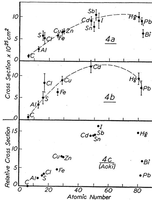
FIG. 4. *a*, Effective absorption cross sections for medium fast neutrons as measured with a Cu detector; *b*, same, measured with a Pb detector; *c*, relative cross sections for the production of gamma-rays by 2.4 Mev neutrons (Aoki).
