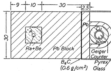
FIG. 3. Experimental arrangement for measuring effective absorption of medium fast neutrons.
