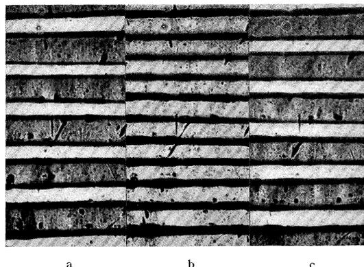
FIG. 3. Patterns of magnetic colloid on a cobalt surface approximately perpendicular to the basal plane with applied normal field (a) outward; (b) zero; (c) inward. The lines run parallel to the hexagonal axis. Magnification approx.  $65\times$ .
