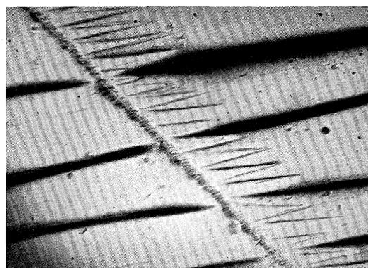
FIG. 6. Pattern of magnetic colloid associated with structure interpreted as a twin band. This pattern was found on the crystal grain which gave Fig. 3. Magnification approx. 215 $\times$ .
