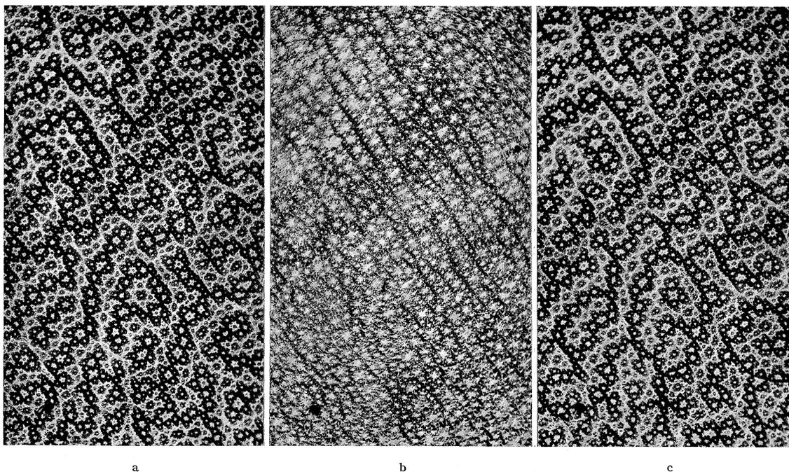
FIG. 2. Patterns of magnetic colloid on the basal plane of a cobalt crystal with applied normal field (a) outward; (b) zero; (c) inward. The spaces and deposits are interchanged in (a) and (c). Magnification approx.  $75\times$ .
