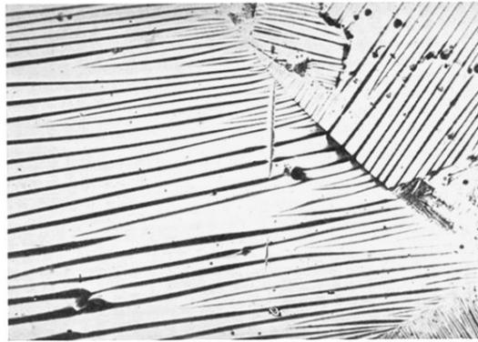
FIG. 4. Line patterns on several crystal grains with no applied field. The lines are spaced closer together in the smaller grains. Lines on adjacent grains tend to join at the grain boundaries. The V shaped line deposits near these boundaries are especially to be noted. Magnification approx. 65 $\times$ .
