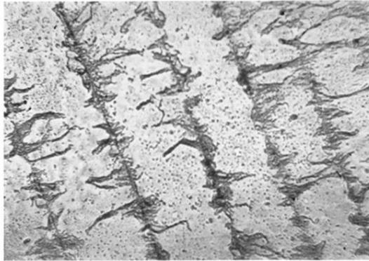
FIG. 1. Distribution of film which was set free from the surface (a prism plane) early in the process of electrolytically polishing cobalt. No applied field. Magnification approx. 215 $\times$ .
