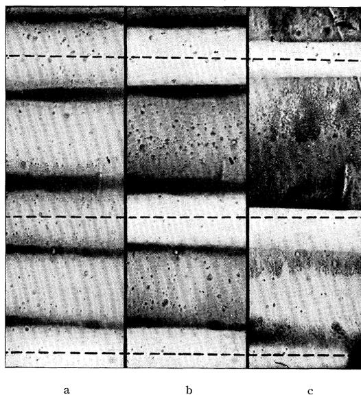
FIG. 5. Set of patterns which illustrate widening of bands when the applied normal field is increased. (a) No field; (b) small applied field; (c) applied field 5 times as intense as in (b). Magnification approx. 190 $\times$ .
