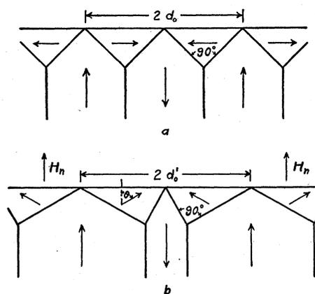
FIG. 7. (a) Schematic diagram (according to Landau and Lifshitz) showing arrangement of magnetization in plane perpendicular to a surface which is perpendicular to direction of easy magnetization. (b) Previous diagram so modified as to include the presence of an applied normal field  $H_n$ . Neither of these arrangements of magnetization demanded by minimum total energy of the crystal gives rise to superficial stray fields which can produce magnetic powder patterns.
