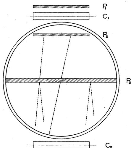
FIG. 1.  $C_1$  and  $C_2$  are Geiger counters;  $P_3$  the shower source;  $P_1$ , 0.36 cm lead;  $P_3$ , 0.36 cm lead.
