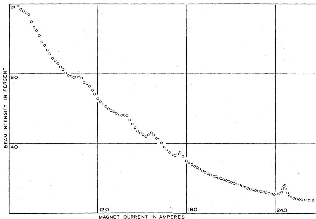
FIG. 7. Detail of the low current part of Fig. 3 showing the peaks arising from the metastable  ${}^2P_{3/2}$  atoms against the background of undeviated  ${}^2P_{1/2}$  atoms.
