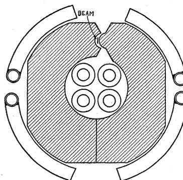
FIG. 2. Cross section of magnet and windings. The beam runs through the curved gap. This diagram is  $\frac{2}{3}$  full size.
