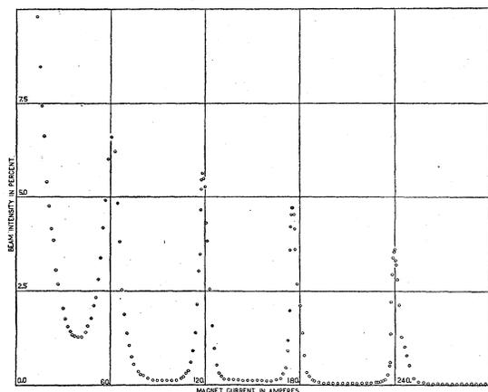
FIG. 3. Plot of the beam intensity against magnet current with detector fixed at the center of the beam.
