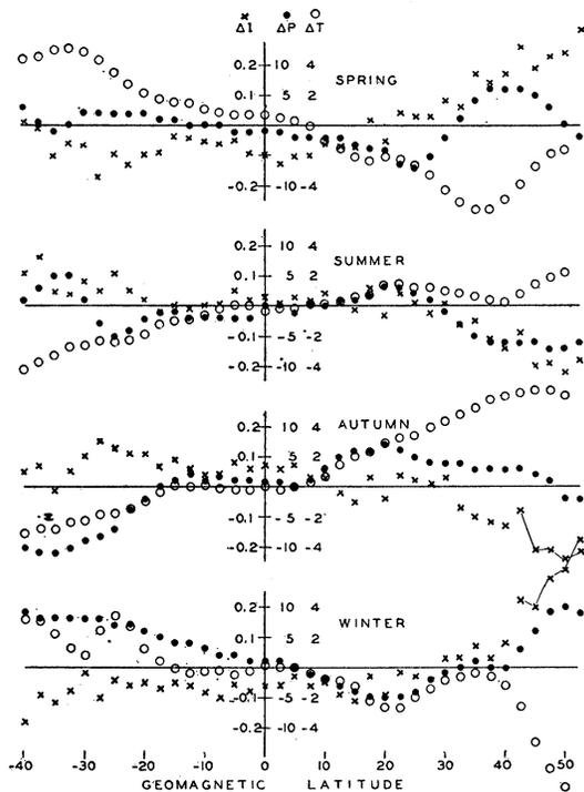
FIG. 8. Seasonal departures from annual mean of ionization ( $\Delta I$ ), argon pressure ( $\Delta P$ , which measures the meter temperature), and shade temperature of the outside air ( $\Delta T$ ), plotted for the various latitudes.
