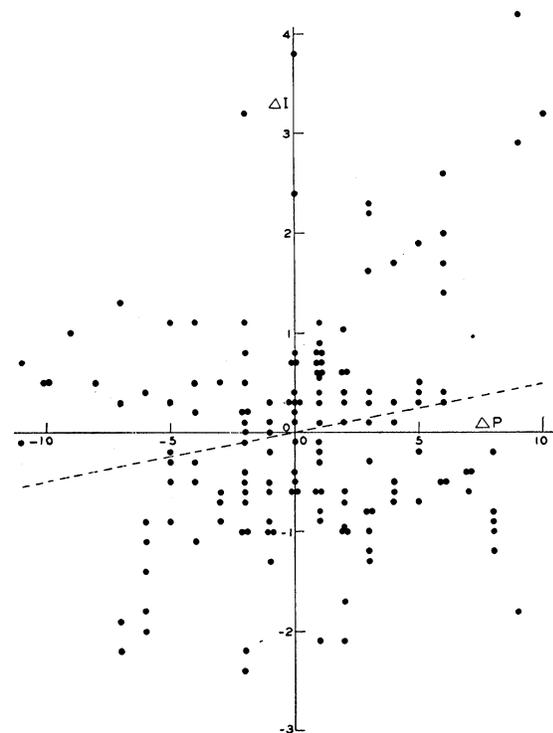
FIG. 9. Scatter diagram of  $\Delta I$  vs.  $\Delta P$ , showing low correlation and negligible temperature coefficient of the meter.
