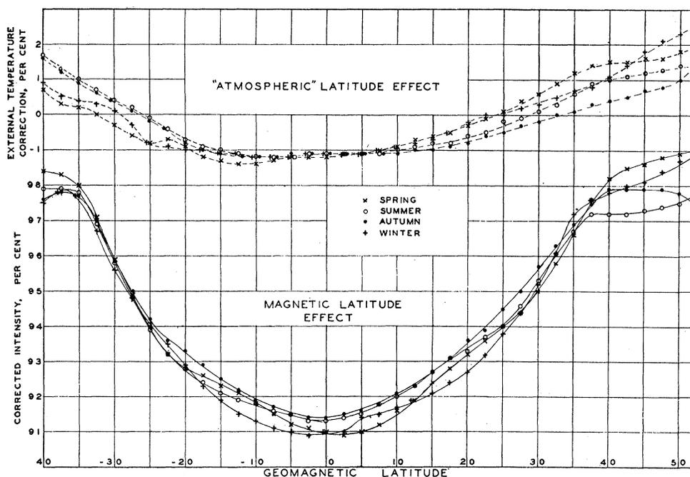
FIG. 10. Magnetic (solid lines) and atmospheric (broken lines) latitude effect for the four seasons. Sum of these two effects gives observed total effect of Fig. 7.
