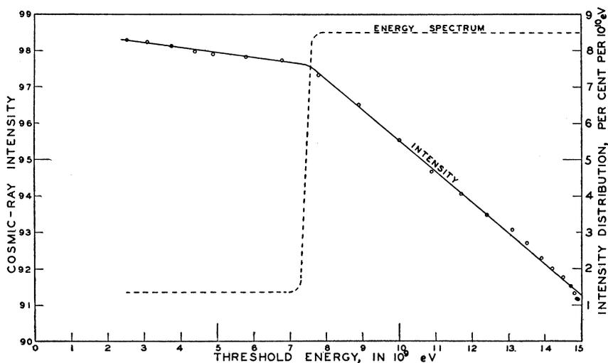
FIG. 13. Solid line, cosmic-ray ionization as function of geomagnetic energy threshold. Broken line, energy distribution of primary cosmic rays, according to geomagnetic analysis.
