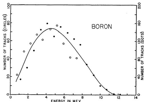
FIG. 4. Experimental spectrum of beta-rays from  $\text{B}^{12}$ . Circles are for 1220 gauss field (right-hand ordinate scale). Dots are for 2440 gauss field (left-hand ordinate scale).
