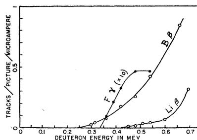
FIG. 8. Excitation curves for the reactions producing the Li and B beta-rays (unresolved ion beam). The voltage scale is calibrated by the excitation curve for the  $\text{F} + \text{H}^1$  gamma-rays. For the beta-rays the solid angle subtended by the chamber window at the source was about  $\pi/4000$ .
