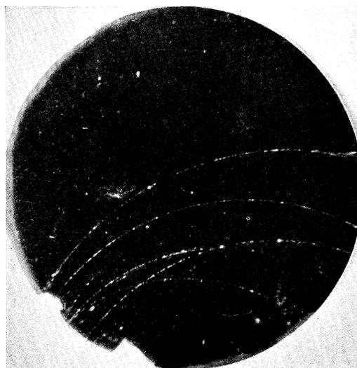
FIG. 2.  $\text{Li}^8$  beta-rays entering the cloud chamber through a thin window. This is the arrangement used for measuring the upper limits of the  $\text{Li}^8$  and  $\text{B}^{12}$  spectra.
