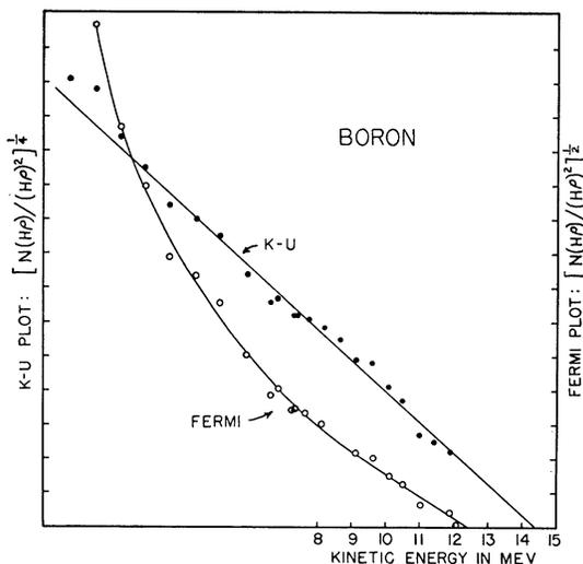
FIG. 6. K-U and Fermi plots for  $\text{B}^{12}$ . These include the separate upper limit data shown in Fig. 5.
