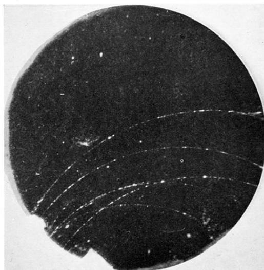
FIG. 2.  $\text{Li}^8$  beta-rays entering the cloud chamber through a thin window. This is the arrangement used for measuring the upper limits of the  $\text{Li}^8$  and  $\text{B}^{12}$  spectra.
