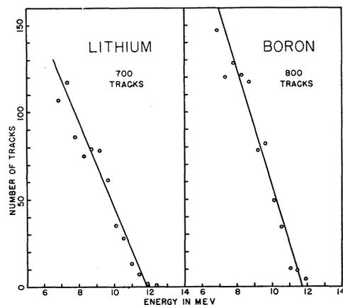
FIG. 5. Plots of separate data obtained near the upper limits of the  $\text{Li}^8$  and  $\text{B}^{12}$  spectra.
