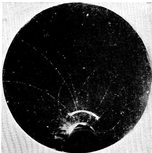
FIG. 1.  $\text{Li}^8$  beta-rays from a thin walled thimble inside the cloud chamber. Three of these tracks satisfy the requirements for measurement.
