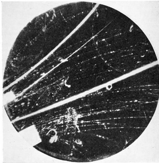
FIG. 7. Protons of the 90 cm range group and electrons from a target of  $B^{10}+B^{11}$  bombarded with deuterons.
