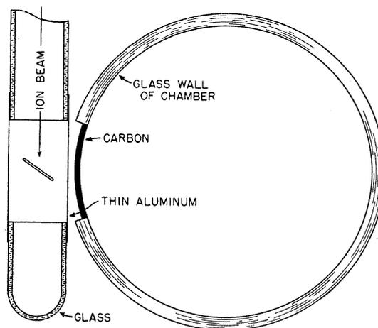
FIG. 2. Vertical cloud chamber arrangement.
