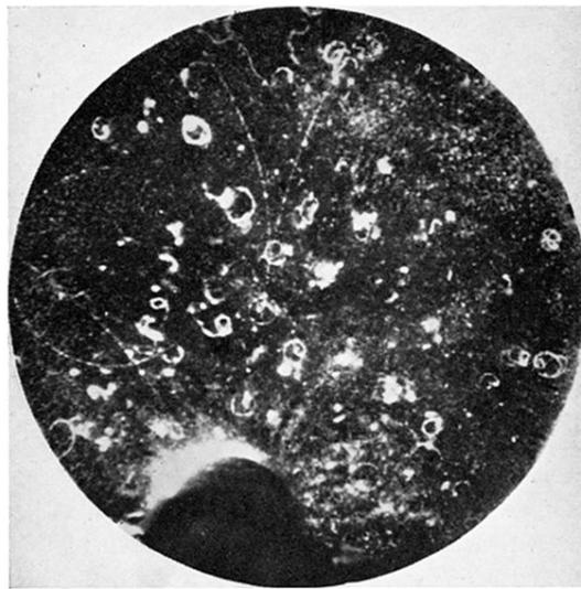
FIG. 9. A pair which originates in the gas in the cloud chamber. Its total energy is 17.1 Mev, with an uncertainty due to measurement and fluctuation in the magnetic field of at least  $\pm 0.5$  Mev. One pair of this kind gives a good approximation to the quantum energy of one of the gamma-ray lines, because it suffers no absorption.
