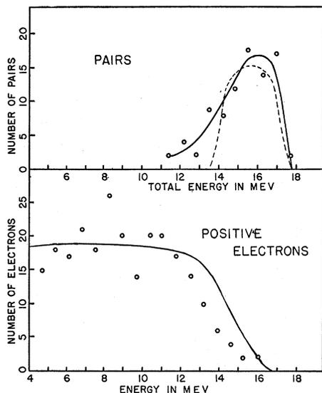
FIG. 7. Upper plot: Pairs ejected from 2 mm carbon by the  $\text{Li-H}^1$  radiation, in the horizontal arrangement.  $H=2350$  oersteds. The dotted curve is the theoretically expected distribution from a 17 Mev gamma-ray line and 2 mm carbon. Lower plot: Positrons which appear singly or as members of pairs. The curve shows the expected distribution from a 17 Mev gamma-ray line.
