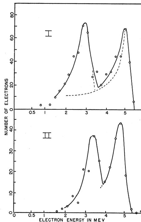
FIG. 10. Negative electrons produced by the gamma-radiation from  $\text{F} + \text{H}^1$ . I: Horizontal arrangement of Fig. 1, 1.5 mm carbon scatterer. II: Collimated gamma-ray beam falling upon a 1.5 mm carbon sheet placed across the center of the chamber.  $H = 1850$  oersteds.
