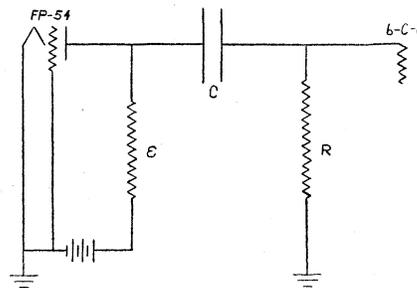
FIG. 2. Diagram for analysis of recording circuit.
