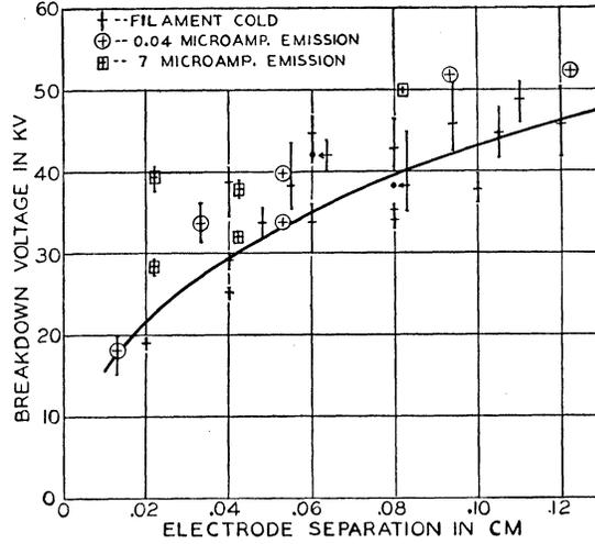
FIG. 1. Breakdown voltage vs. electrode separation, with cathode cold and with cathode heated to give different electron emission (measured at 200 volts). Solid curve shows voltage necessary to produce a constant field of 600 kv per cm at the cathode.
