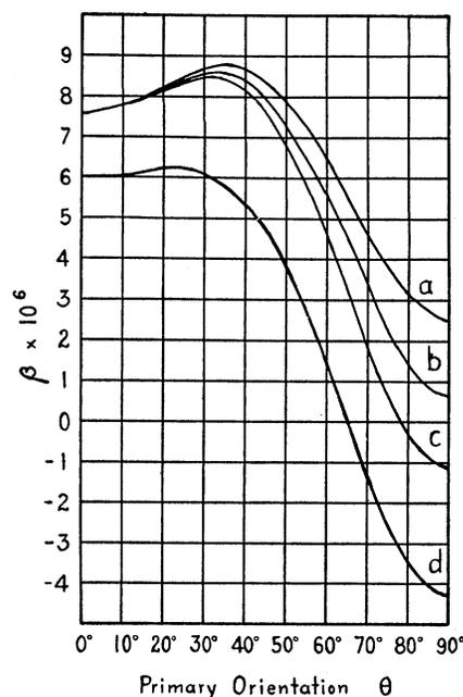
FIG. 2. Tension coefficients of tin directly observed: *a*,  $\varphi=45^\circ$ ; *b*,  $\varphi=22\frac{1}{2}^\circ$ ; *c*,  $\varphi=0^\circ$ . Coefficients of specific resistance—curve *d*.
