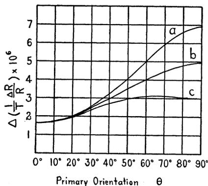
FIG. 1. Relative change of resistance per unit tension due only to changes in dimensions and orientation and computed from Bridgman's determination of the elastic constants of tin. *a*,  $\varphi = 45^\circ$ ; *b*,  $\varphi = 22\frac{1}{2}^\circ$ ; *c*,  $\varphi = 0^\circ$ .
