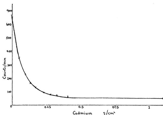
FIG. 3. Absorption of neutrons in cadmium.
