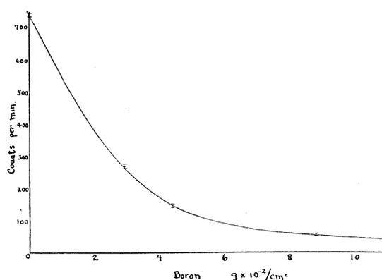
FIG. 2. Absorption of neutrons in Pyrex plates.
