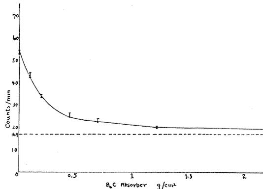
FIG. 4. Absorption of neutrons in  $\text{B}_4\text{C}$  filtered through  $0.582 \text{ g/cm}^2 \text{ Cd}$ .
