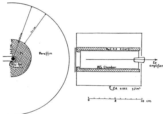
FIG. 1. Arrangement of source and ionization chamber.
