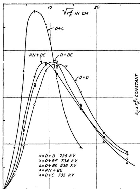
FIG. 10. Thermal neutrons in water between successive spherical shells (ordinates adjusted to give equal areas under curves).
