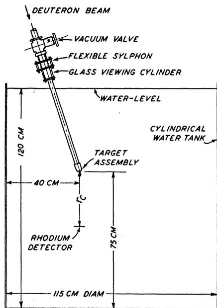
FIG. 1. Arrangement of target and water tank.
