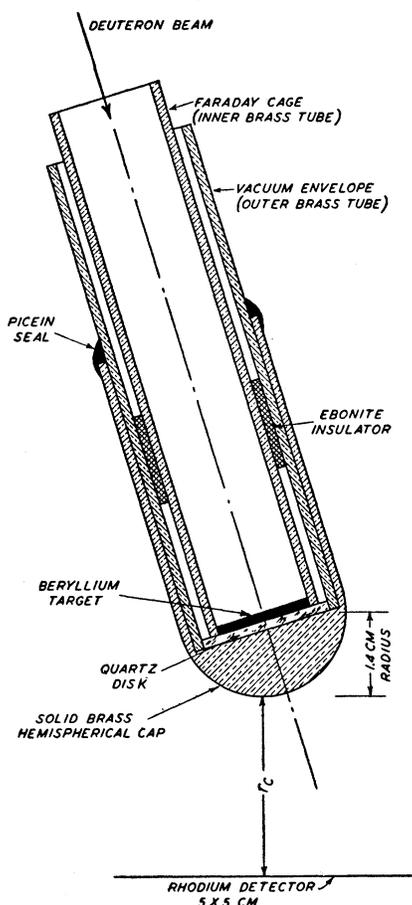
FIG. 2. Detail of target assembly.
