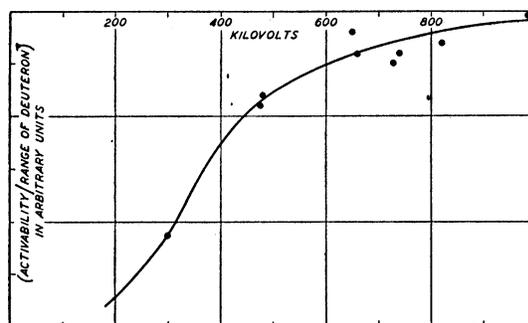
FIG. 8. Efficiency curve for  $D+D$  reaction.
