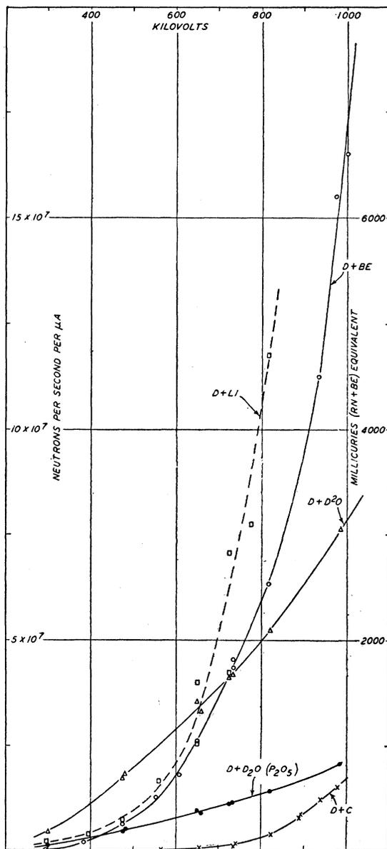
FIG. 9. Total neutron yields at various voltages for several deuterium reactions. (Multiply curve for  $D+D_2O$  by 0.93.)
