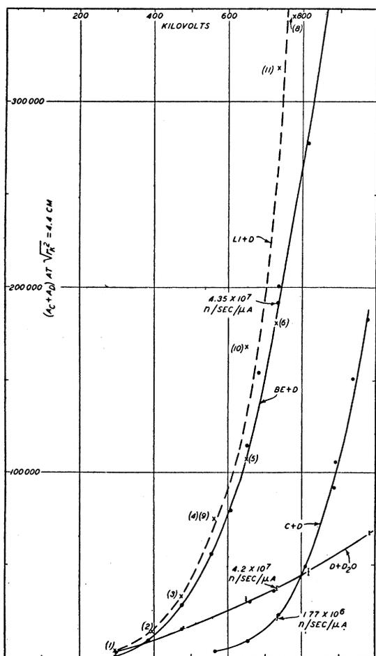
FIG. 7. Thermal neutrons at fixed distance, source at various voltages, for several deuterium reactions. (For absolute yield multiply curve for  $D+D_2O$  by 0.93.)
