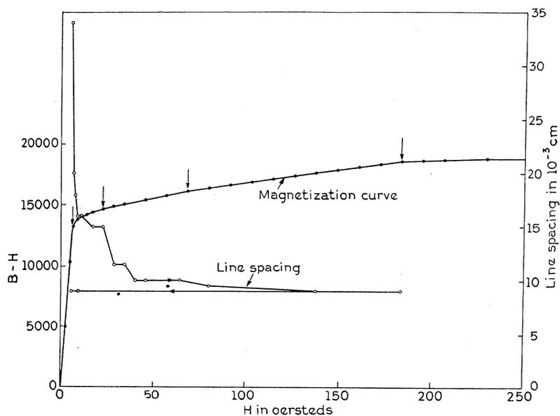
FIG. 4. Magnetization curve of crystal No. 7N (not corrected for demagnetizing effect) and line spacing (Type II) vs. field relation. The vertical arrows point to sharp breaks in the magnetization curve.
