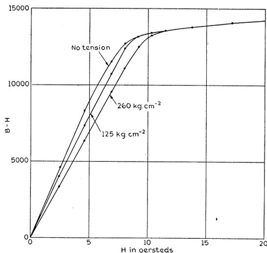
FIG. 5. The first part of the magnetization curve of crystal No. 7N with different values of tension.
