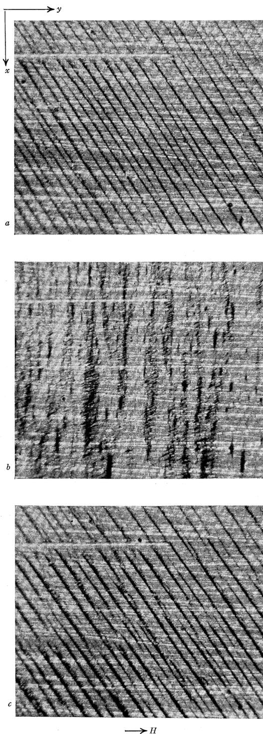
FIG. 3. *a*; Pattern (Type II) on crystal No. 70 at 36 oe. *b*; Pattern (Type III) after the field was raised to 90 oe. *c*; Pattern (Type II) after field reduction from 90 to 35 oe. (Magnification 15 $\times$ .) The Type II field range on crystal No. 70 lay between 8 and 80 oe.
