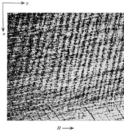
FIG. 1. Type I pattern on crystal No. 70 at 5 oe. Due to inhomogeneous field distribution, several Type II lines appear on the lower part of the figure. The white lines are polishing scratches. (Magnification 15 $\times$ ).
