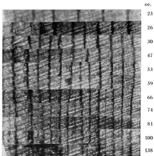
FIG. 2. Type II patterns taken at the same place on crystal No. 1 after successive increases in field. (Magnification 48 $\times$ .) The Type II pattern on crystal No. 1 was observed in a field range between 20 and 160 oe.
