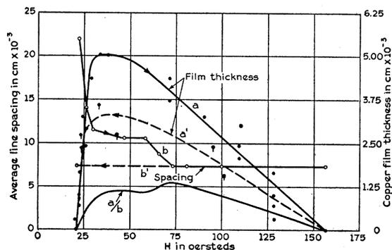
FIG. 6. Copper film thickness, at which the Type II pattern disappears, and spacing on crystal No. 1.
