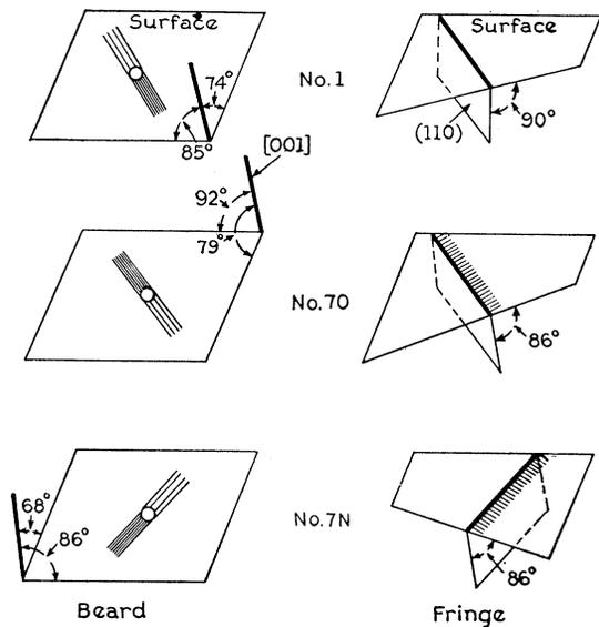
FIG. 8. The direction of "beards" caused by a hole and of "fringes" forming on lines, for different crystals.
