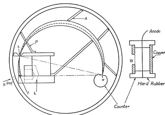
FIG. 1. Diagram of spectrograph with counter.
