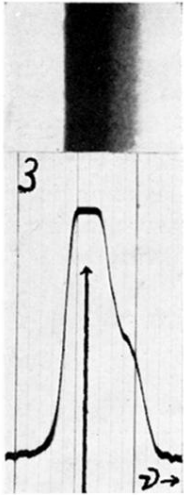
FIG. 3. Tl 3775.7, 10 cm A. There is a narrow band on the short wave-length side of the line, relative intensity 1/350.
