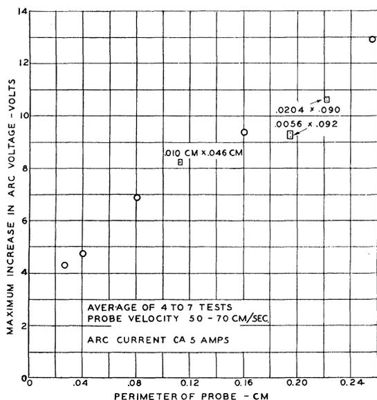
FIG. 2. Increase in arc voltage caused by probe swinging through arc.
