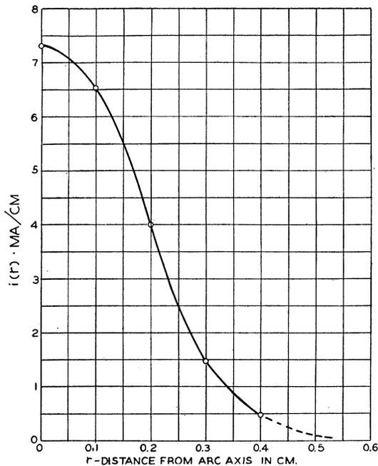
FIG. 9. Positive ion current collected per cm length of probe.
