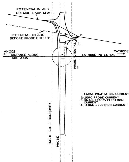
FIG. 7a. Potential distribution around probe.
