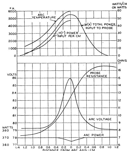
FIG. 4. Thermal probe in arc.
