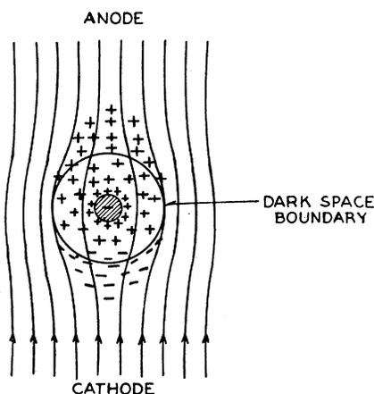
FIG. 7b. Space charges and lines of current flow around probe. Section perpendicular to probe.
