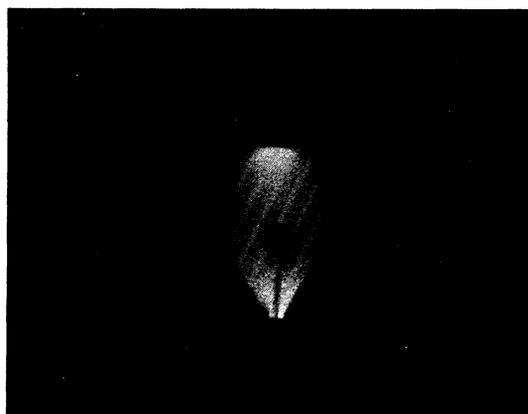
FIG. 3. Photograph of 6-amp., 0.89 cm long, arc with 0.025 cm probe wire 0.38 cm from cathode (lower) electrode.
