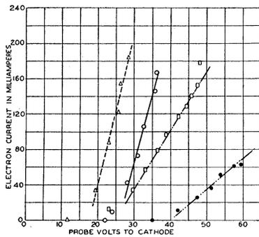
FIG. 6a. Probe current voltage characteristics. Triangle, probe 0.13 cm from cathode, arc 6 amp.; open circle, probe 0.38 cm from cathode, arc 8.7 amp.; square, probe 0.38 cm from cathode, arc 5.9 amp.; closed circle, probe 0.38 cm from cathode, arc 3.2 amp.
