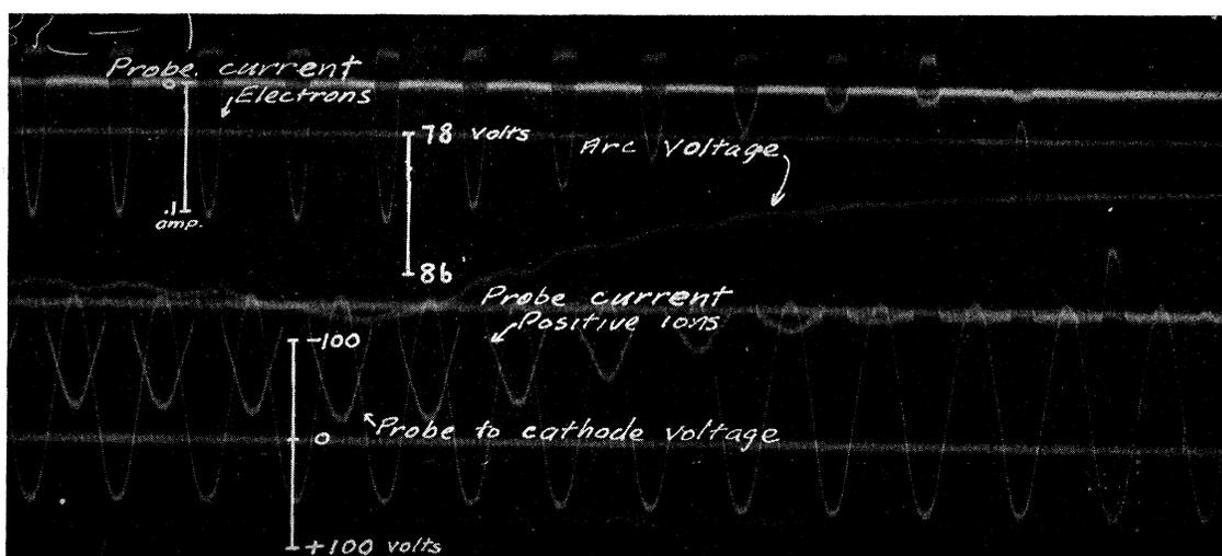
FIG. 5. Probe 0.51 cm from cathode of 6-amp., 1.14 cm long, arc. Probe moved through arc during exposure of film.
