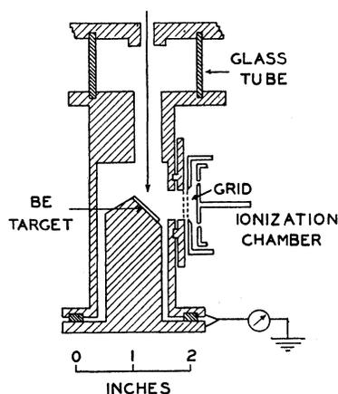
FIG. 1. The target assembly and ionization chamber.
