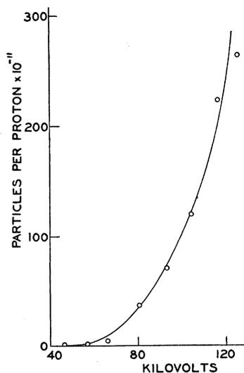
FIG. 3. The excitation curve for a thick target of beryllium. Thyatron grid bias set for the recording of both groups of particles.
