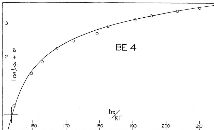
FIG. 5. Fowler plot for Be. elec./quant.,  $\phi = 3.92$  V.
