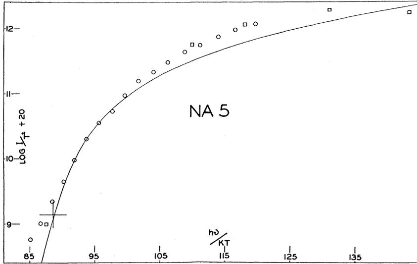
FIG. 6. Fowler plot for Na.  $\phi = 2.29$  V.
