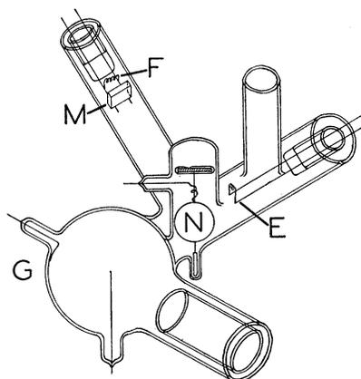
FIG. 2. Magnesium photo-cell.
