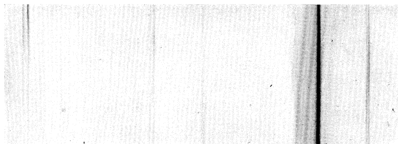
FIG. 3. Typical spectrogram. From left to right, Cu K\alpha , Zn K\alpha , Cu K\beta_1 , Zn K\beta_1 , and Va K\alpha in the first order. Enlargement about 3X. Ghost structure on long wave-length side of Zn K\beta_1 . Zn K\beta_2 , \gamma was visible on the original negative. Obtained from ZnS.
