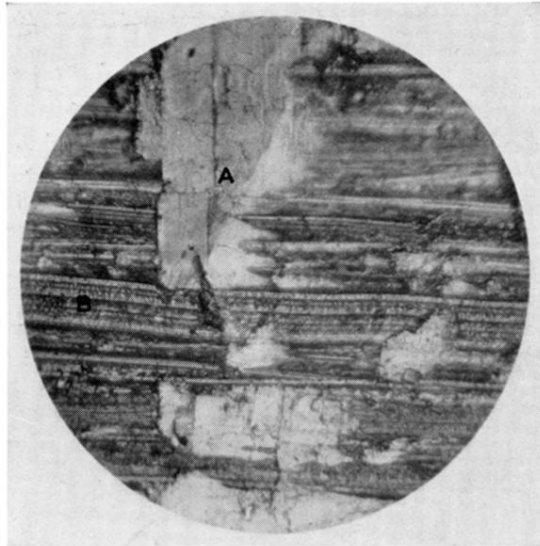
FIG. 1. Cube face of a galena crystal which has been filed from left to right, parallel to a cube edge. Magnification 90X.
