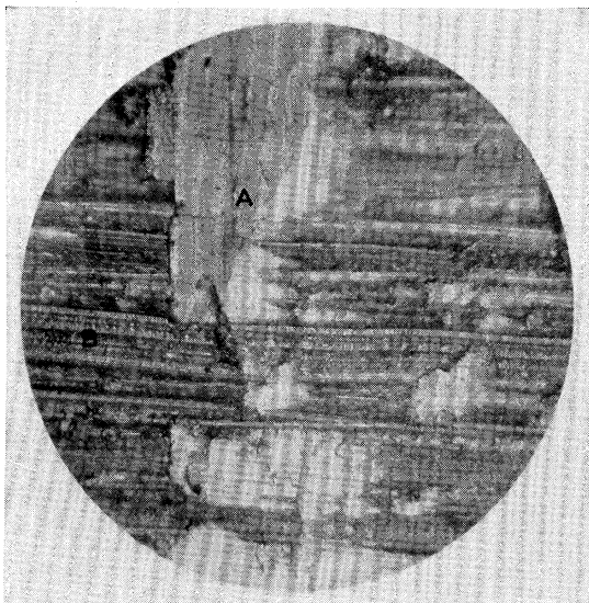
FIG. 1. Cube face of a galena crystal which has been filed from left to right, parallel to a cube edge. Magnification 90 \times .
