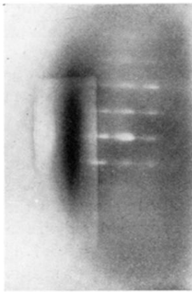
FIG. 2. Electron diffraction pattern from such a mirror surface of galena as that marked A in Fig. 1. Surface brushed to remove powdered galena, but not etched. Primary beam nearly parallel to a cube edge.
