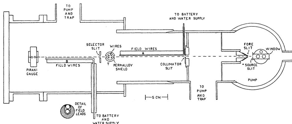
FIG. 3. Diagram of apparatus as used for determination of the sign of the moment for hydrogen and deuterium. The permalloy shield and the wires *T* were removed from the apparatus for the measurement of the magnitudes of the moments.
