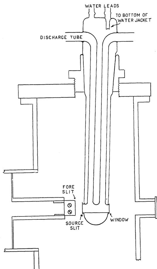
FIG. 4. Section of source chamber to show the construction of discharge tube and of the eccentric brass adjusting collar.
