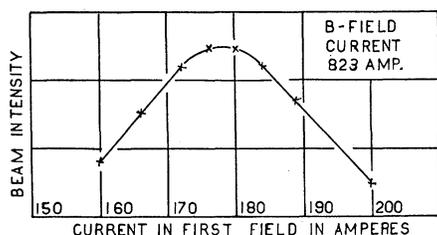
FIG. 6. Intensity of beam against field with selector slit interposed to pass only atoms with negative moments, for hydrogen.
