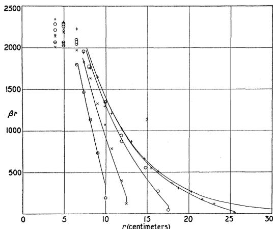
FIG. 2. Plots of  $\beta r$  vs.  $r$  for the indium detector in spheres of radii 10, 12.5, 17.55, and 25.55 cm, respectively, from left to right. The curves for the spheres of various radii were drawn using Eq. (5). The top curve is for a sphere of infinite radius.
