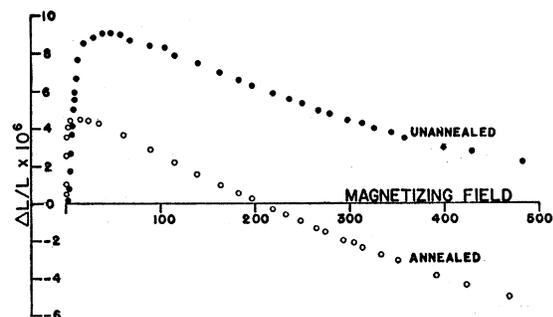
FIG. 4. The longitudinal magnetostriction of unannealed and annealed Armco iron.
