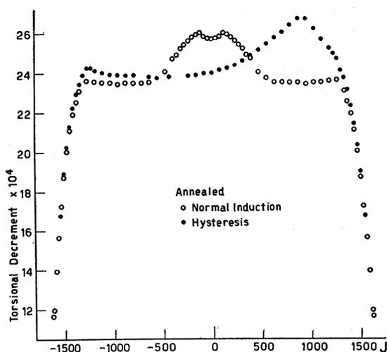
FIG. 3. Variation of the torsional decrement with magnetization in annealed Armco iron.
