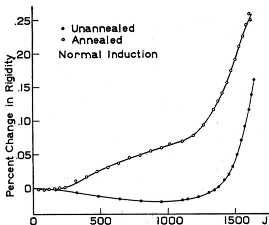
FIG. 1. Variation of the rigidity modulus with magnetization in unannealed and annealed Armco iron.
