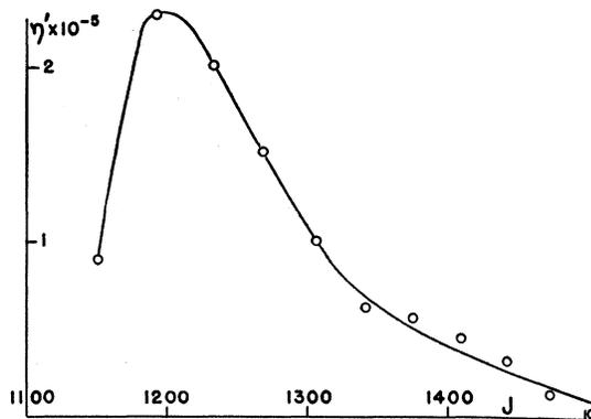
FIG. 5. The Wiedemann effect in annealed Armco iron.
