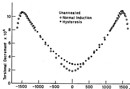
FIG. 2. Variation of the torsional decrement with magnetization in unannealed Armco iron.
