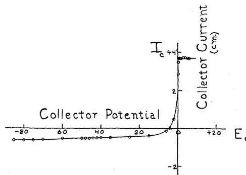
FIG. 3. Current-voltage curve for the collector for 625-volt ions. (Cold target.)
