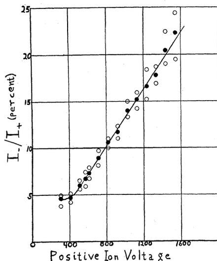
FIG. 5. Variation of the secondary electron emission from the hot target with the positive ion voltage. Average values ( $\bullet$ ), extreme values ( $\circ$ ).
