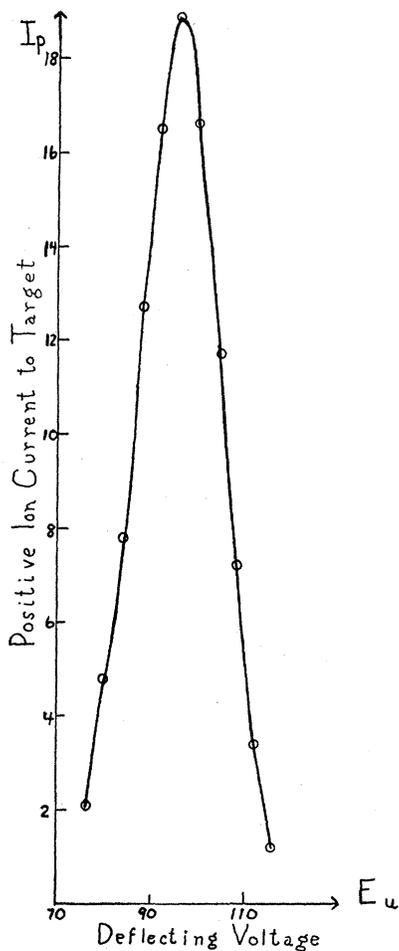
FIG. 2. Curve showing how the positive ion current to the target varies with the deflecting voltage for 855-volt ions.
