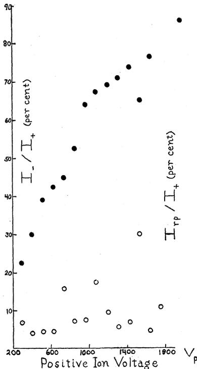
FIG. 4. Variation of the number of secondary electrons (●) and of reflected positives (○) per positive ion with positive ion voltage for a cold target.
