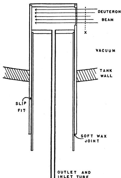
FIG. 1. Experimental arrangement used for activating argon with deuterons. For activation with neutrons, a beryllium target is introduced at X.
