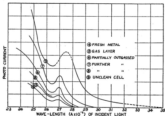
FIG. 2. Characteristic of cell containing evaporated aluminum film.
