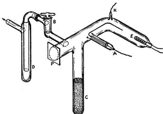
FIG. 1. Photoelectric cell.
