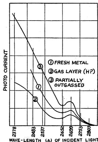
FIG. 3. Characteristic of cell containing evaporated aluminum film.
