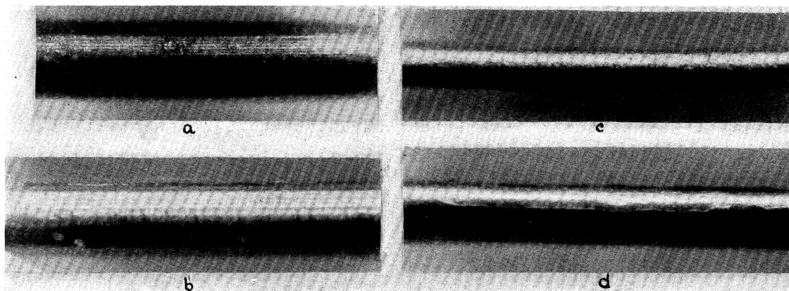
FIG. 4. Microphotographs of tungsten filament surfaces. (a) Raw wire from spool; (b) piece of same wire after about one hour at 2800°K; (c) wire smoothed by electrolysis; (d) piece of same wire after about one hour at 2800°K.
