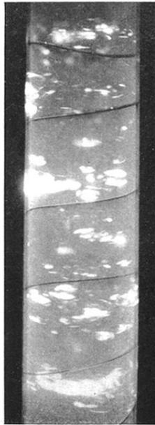
FIG. 2. Cold emission from a raw tungsten wire.
