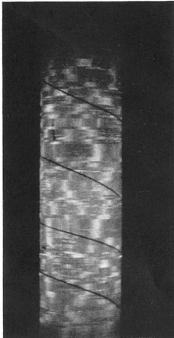
FIG. 9. Cs-W pattern at  $\sim 800^{\circ}\text{K}$ , showing the degree of recrystallization produced by several flashes to  $3100^{\circ}\text{K}$ . (G. E. 218 wire, smoothed by abrasion.)
