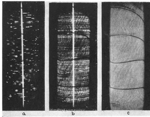
FIG. 5. Typical patterns of thoriated tungsten ( $1200^{\circ}\text{K}$ ). (a) immediately after flash to  $2800^{\circ}\text{K}$ ; (b) after first 4 minutes of activation at  $1850^{\circ}\text{K}$ ; (c) after 40 minutes of activation at  $1800^{\circ}\text{K}$ .
