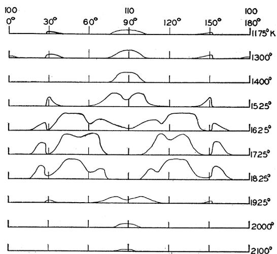
FIG. 8. Influence of preparation temperature on single-crystal patterns at  $\sim 775^\circ\text{K}$ . Filament in equilibrium with saturated potassium vapor at  $220^\circ\text{C}$ ; preparation temperatures at right. The curves, sketched during observation, show dependence of emission on angle around a semi-circumference of the tube with the 100 axis as diameter.
