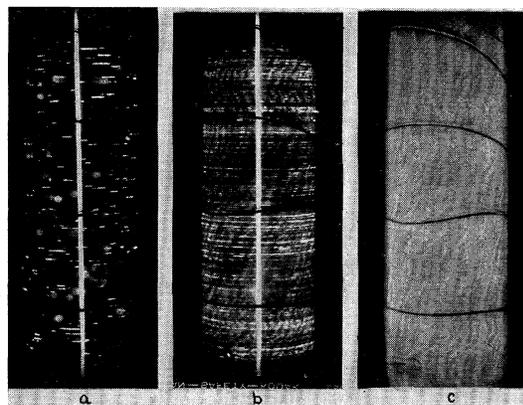
FIG. 5. Typical patterns of thoriated tungsten (1200°K). (a) immediately after flash to 2800°K; (b) after first 4 minutes of activation at 1850°K; (c) after 40 minutes of activation at 1800°K.
