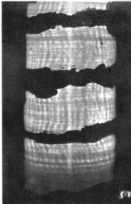
FIG. 3. Emission pattern of a drawn tungsten wire. In this tube the nickel helix was replaced by one of platinum paint.
