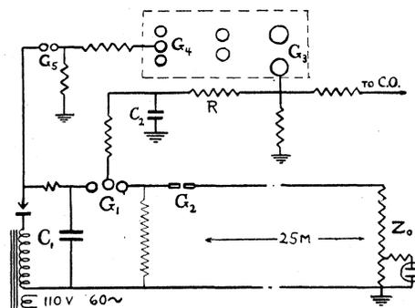
FIG. 6. Circuit for synchronization of the sixty-cycle discharge studied at  $G_2$ .
