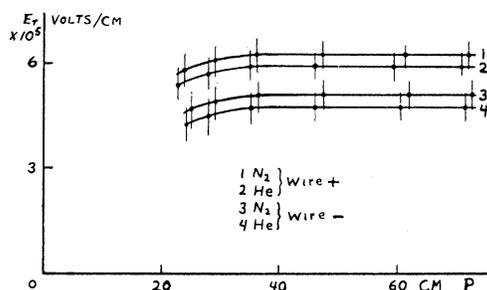
FIG. 2. Overvoltage breakdown intensity-pressure relations between a wire and a concentric cylinder by using circuit in Fig. 1.
