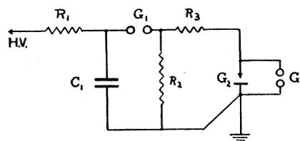
FIG. 1. Circuit for applying potential rapidly to a gap,  $G_2$ , to be overvolted and gap,  $G_3$ , for measuring potential.
