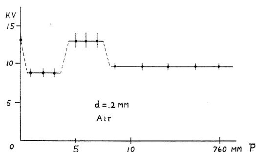
FIG. 5. Overvoltage breakdown potential-pressure relations between 2.5-cm brass spheres as determined by the oscillograph.
