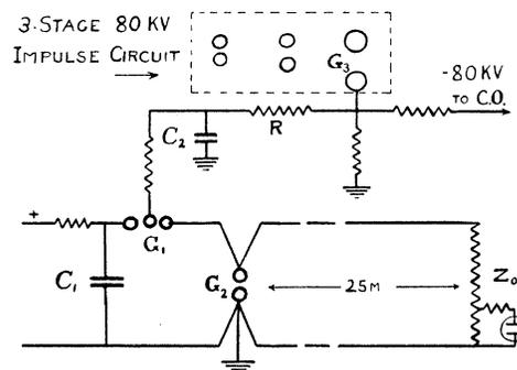
FIG. 3. Circuit for synchronization of the discharge to be studied at  $G_2$  with the oscillograph.
