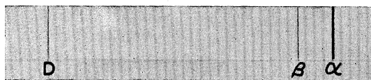
FIG. 1. D is the direct beam, \beta and \alpha the refracted beams of the copper K series.
