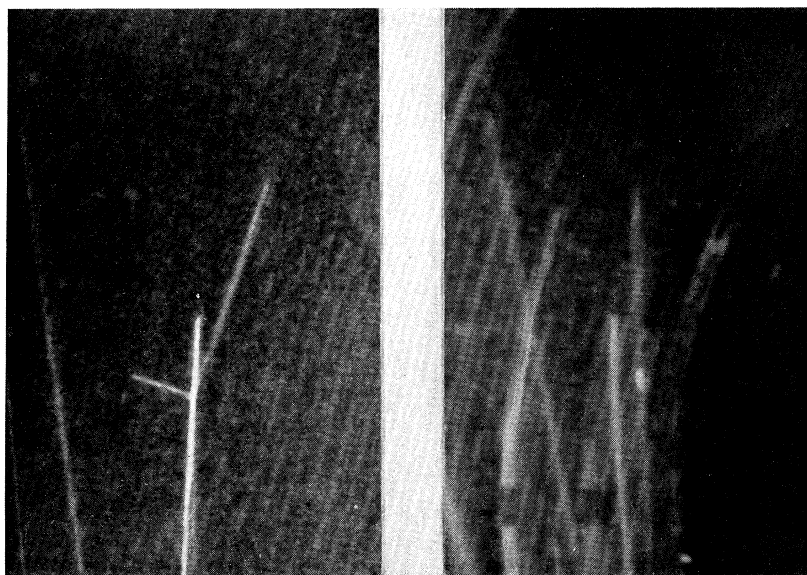
FIG. 5. A proton-proton collision of high energy-exchange, the longer spur being of 3-cm length in the chamber; the plane of the collision contains the axis of one of the camera lenses.
