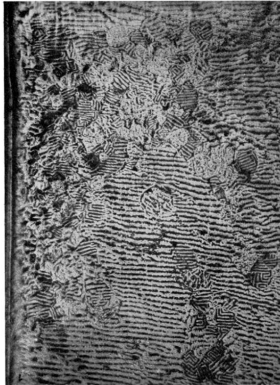
FIG. 9. Colloid concentration pattern for a section of the disk of silicon sheet steel furnished by N. P. Goss. The rolling direction is along the scratch on the left side of the pattern.
