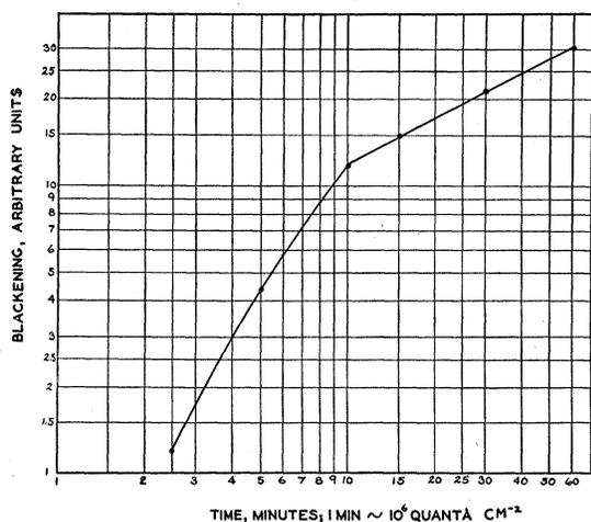
FIG. 3. Blackening of film exposed to x-rays.
