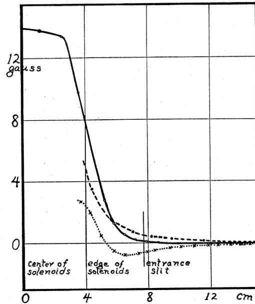
FIG. 5b. Straying of magnetic field due to separation of solenoids. Dashed line, field without compensating coils; dotted line, field due to compensating coils; solid line, field due to solenoids and compensating coils together.
