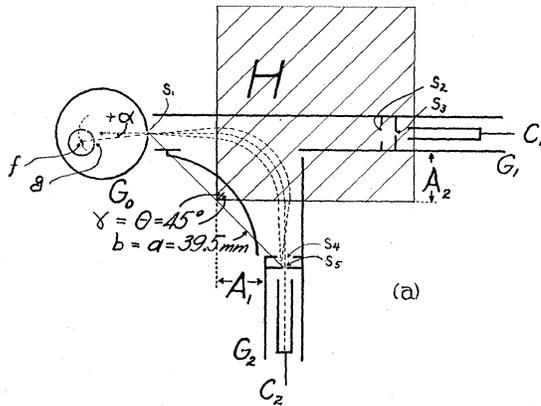
FIG. 3a. Diagrammatic cross section of apparatus for securing refocussing at  $\theta = 45^\circ$ ,  $\gamma = 45^\circ$ .
