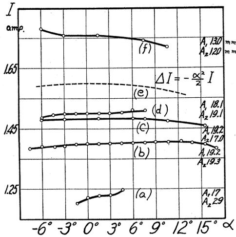
FIG. 4. Experimental test of spread. Dotted line, theoretical; solid lines, experimental ( $I, \alpha$ ) curves for different positions of solenoids.
