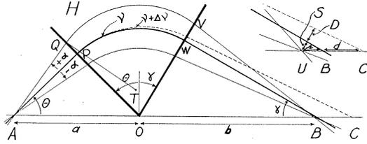
FIG. 1. Refocussing of electron paths. Offset shows region near  $B$  enlarged.
