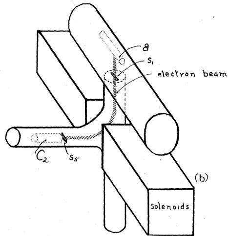
FIG. 3b. Perspective view of apparatus, showing arrangement of the solenoids.
