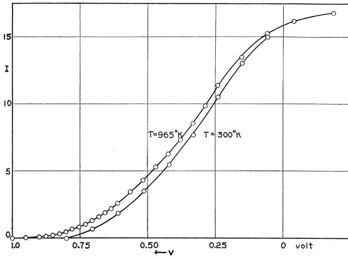
FIG. 3. Observed current-voltage curves for  $\lambda 2400$ .
