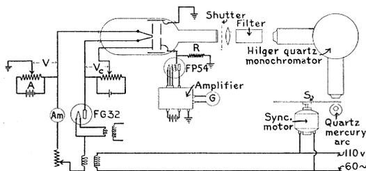
FIG. 2. Wiring diagram. *A*, potential divider. *V*, applied retarding potential. *V<sub>c</sub>*, compensating potential.  $R = 3.9 \times 10^{11}$  ohms. Filter eliminates scattered light of short wave-length.
