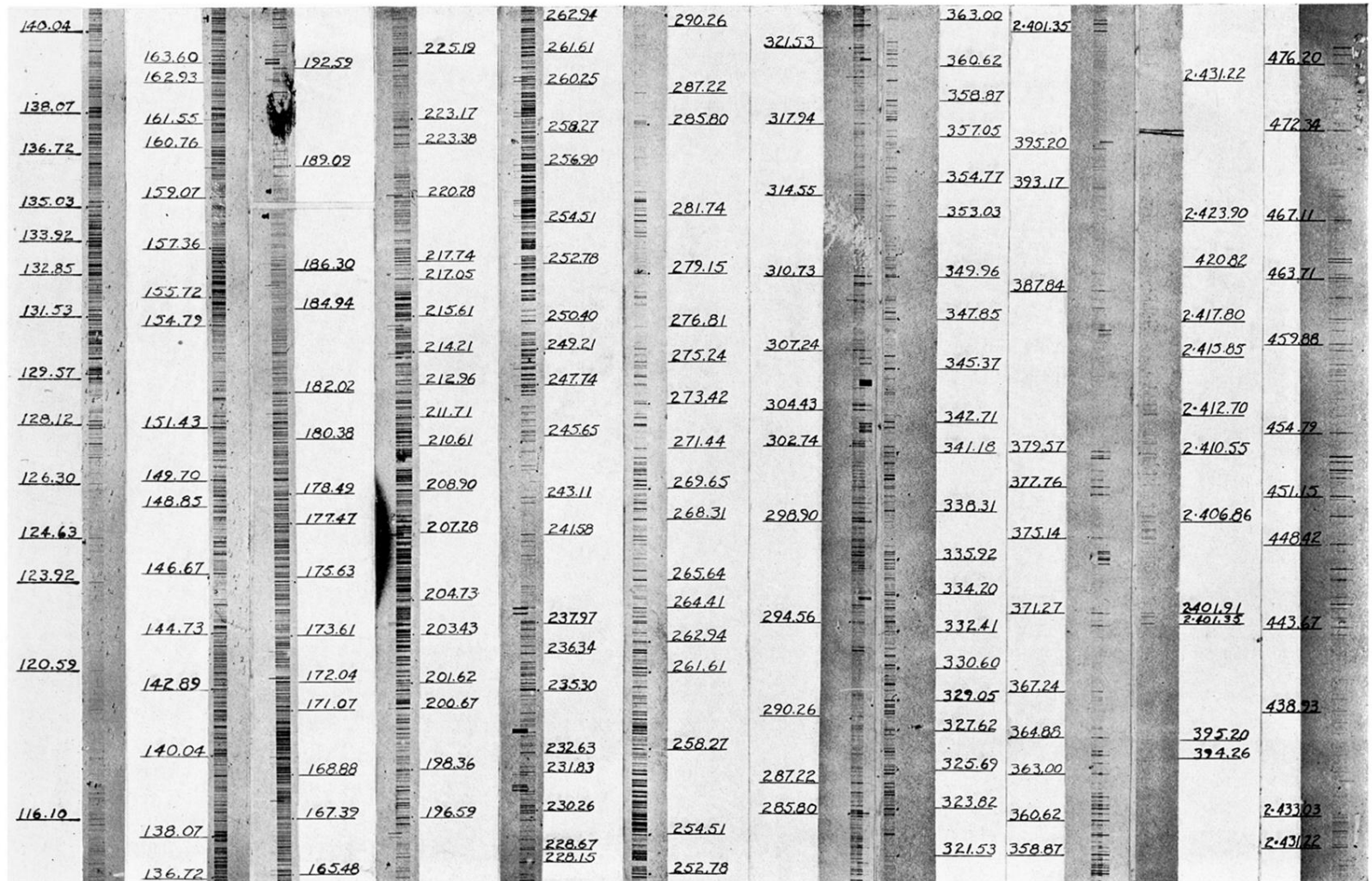
FIG. 1. The copper spectrum with standard lines indicated. Overlapping spectra are due to oxygen, aluminum, and boron.
