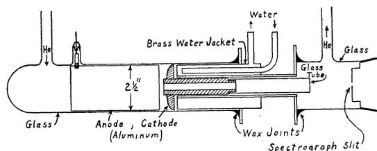
FIG. 1. Discharge tube.
