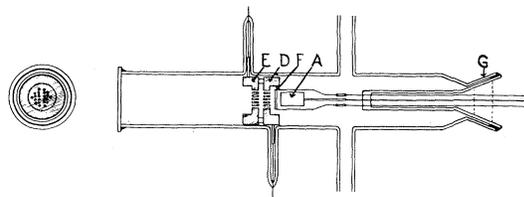
FIG. 1. Discharge tube for production of beams of positive ions of uniform energy.
