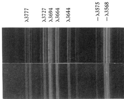
FIG. 2. Doppler effect spectra of neon canal rays, 26,350 and 9100 volts.
