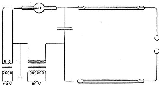
FIG. 3. Diagram of system for illumination of chamber.
