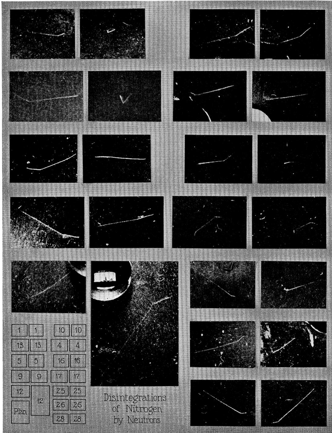
FIG. 5. Paired stereoscopic views of disintegration of nitrogen (by capture of neutron: 1, 13, 5, 9, 12, 10, 4, 16, 17: by scattered neutron: 25, 26, 28).
